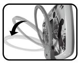
1. Hold the rim vertically and slide it down into the backboard as shown. Then rotate it away from the backboard until you hear it click into place.
